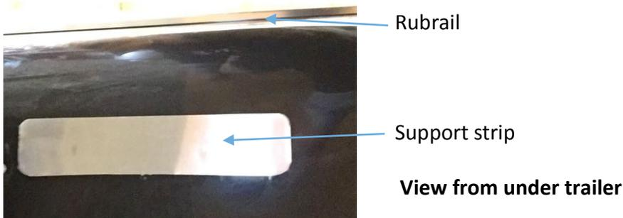
Measure the distance between the support brackets on the hose carrier tube and then mark for inboard metal support strip. You will want the tube brackets to be in the center of support strip.
