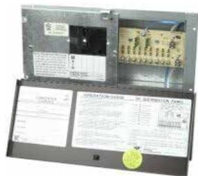
The Parallax 7300 series power center model 7355A had a single stage converter with an output of 55 amps. The battery charging portion will charge the batteries at 13.6 to 13.8 volts.
