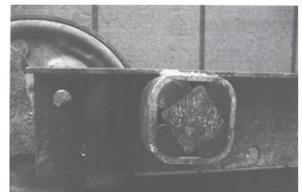
One last point, small trailers (Caravels, Bambi, and others) in the early sixties had five lug wheels and a smaller wheel spindle. They have broken as seen in Figure 2. Don't take the risk. Replace the axle if it has a five lug wheel.
