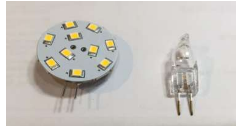
LED replacement -----10W Halogen Bulb 15751w-09 511297-100
