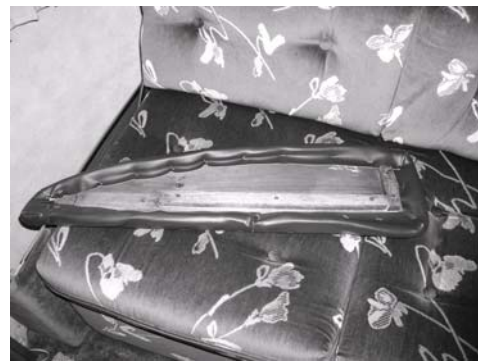
L shaped cleat on bottom of arm holds the arm in place - size and position match original factory arm.
